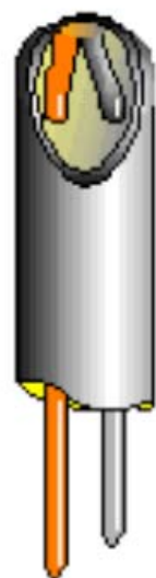
Sealed and Grounded to Sheath
